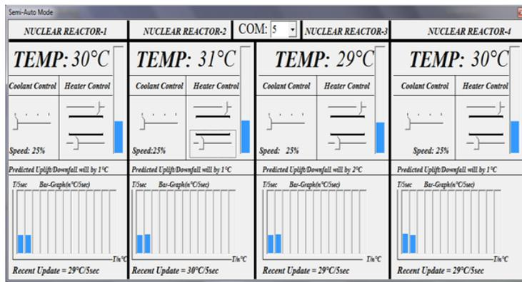
Fig 7: Semi-Auto operating mode form to monitor and control the activities of four nuclear reactors by instructing the software only once and then AI works under FL.
