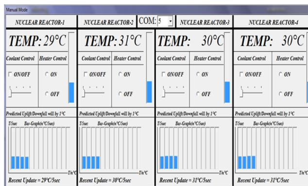
Fig 6: Manual operating mode form to monitor and control the activities of four nuclear reactors manually.
