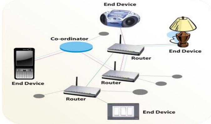
Fig. 1: Zigbee Coordinator (ZC), Zigbee Router (ZR), Zigbee End Devices (ZED).
