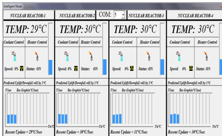
Fig 8: Intelligent operating mode form to monitor and control the activities of four nuclear reactors totally from software’s intelligence by AI under FL by sensing incoming readings.
