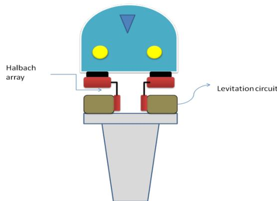
Fig 3. Inductrack model
