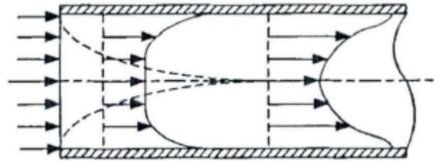
Fig. 1 Temperature distribution in the channel
