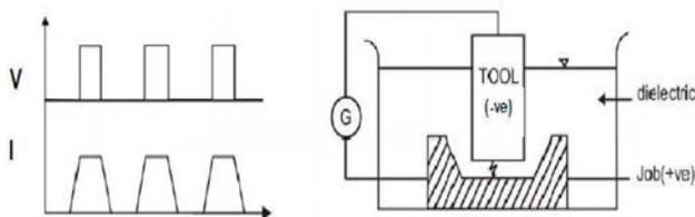
**Figure 2 Working Principle of EDM Process**
