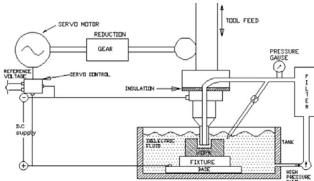
**Figure 1 Set up of Electric Discharge Machining**
