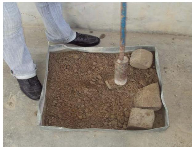
Fig. 1 Crushing of bricks using a Proctor hammer
