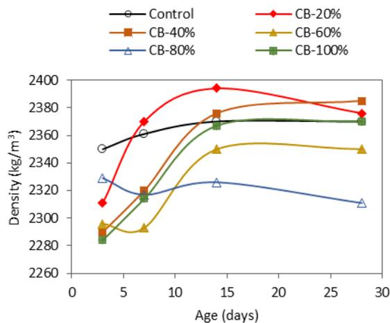
Fig. 4 Variation of density of concrete with age of curing
