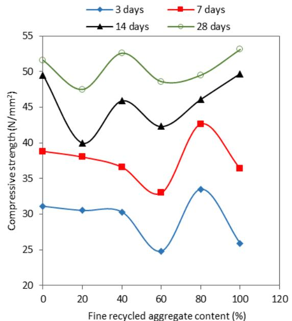
Fig. 6 Compressive strength for varying FRA content
