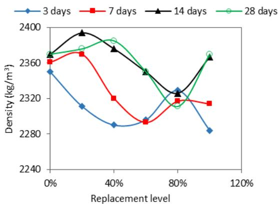
Fig. 3 Effect of crushed bricks content on density of concrete
