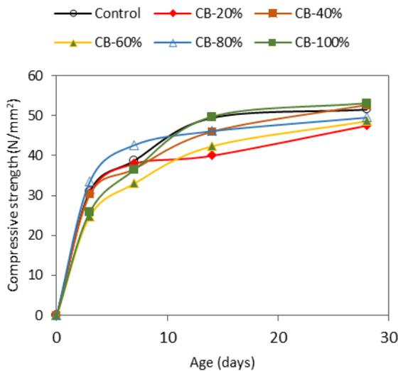
Fig. 5 Variation of compressive strength with age of concrete
