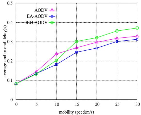
Figure9. node mobility rate  $v_s$  the average end to end delay
