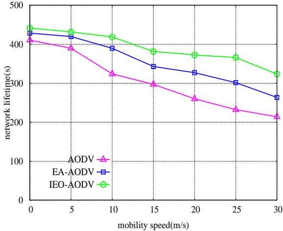
Figure7. node mobility rate  $v_s$  packet network lifetime
