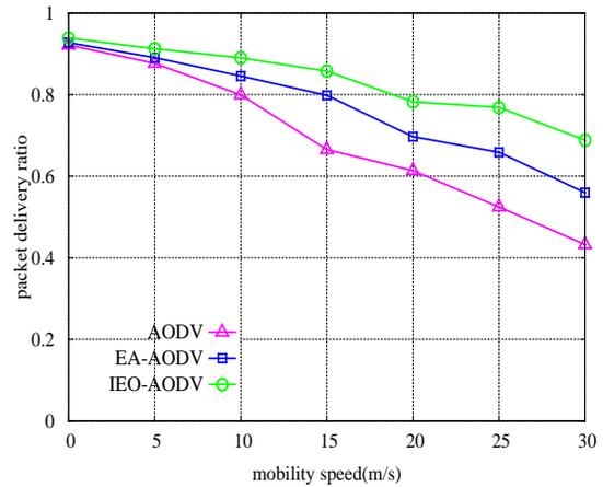
Figure6. node mobility rate vs packet delivery ratio
