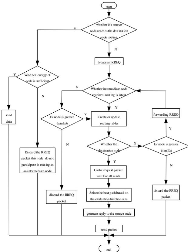
Fig2. IEO-AODV routing protocol establish process
