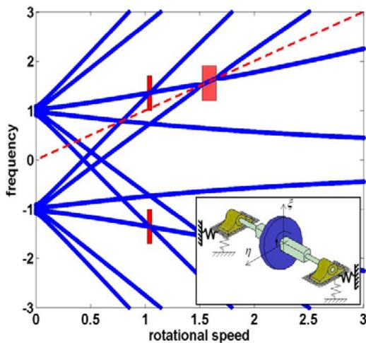
Figure 2 Conventional Campbell diagram for the simple general rotor [4]
