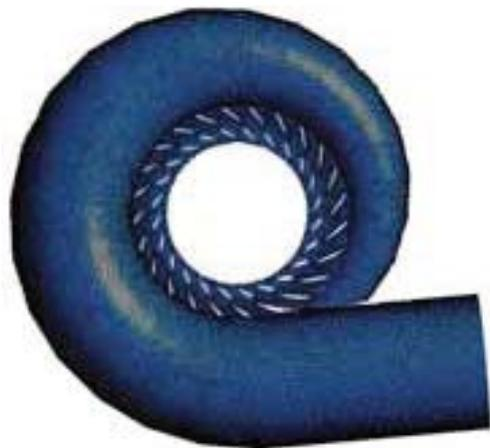
Figure 4 finite element model of spiral casing.
