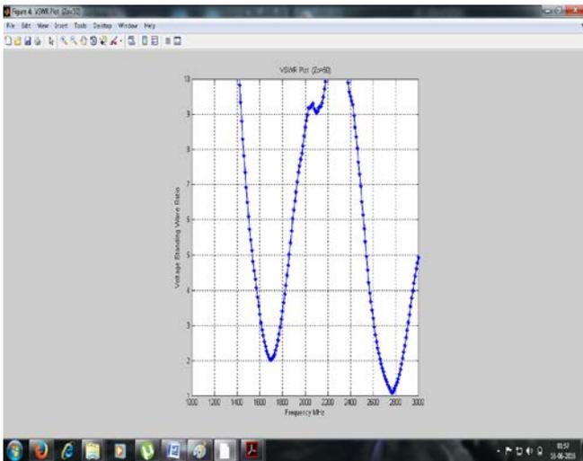
**Figure 6:** VSWR plot of L-Shaped Slot Microstrip Patch Antenna.
