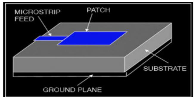
**Figure 1:** Physical Geometry of Microstrip Antenna.
