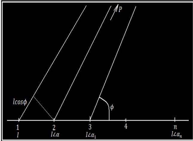
Figure 3: Uniform Linear Array of n Elements.
