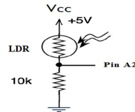
Figure (4) Light sensor circuit
