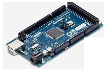
Figure.5 Arduino Mega 2560
