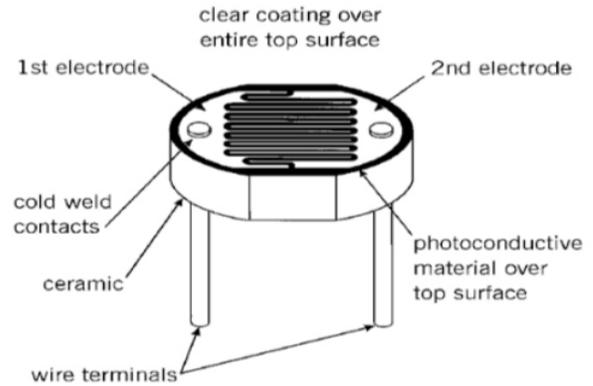
Figure (3) Light Dependent Resistor (LDR)
