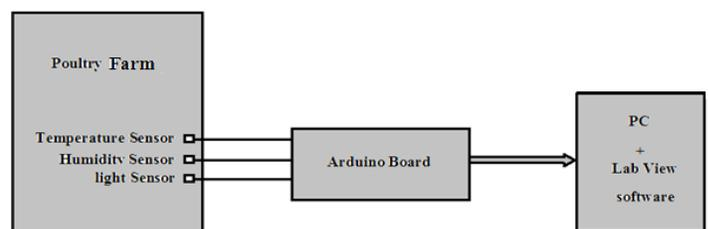
Figure (1): Embedded system architecture
