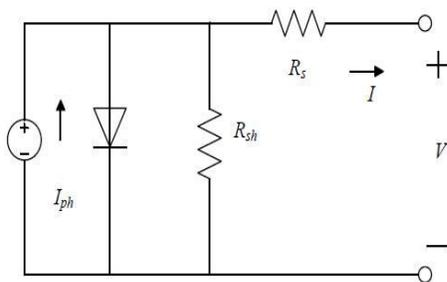
Fig. 1 PV Circuit Model
