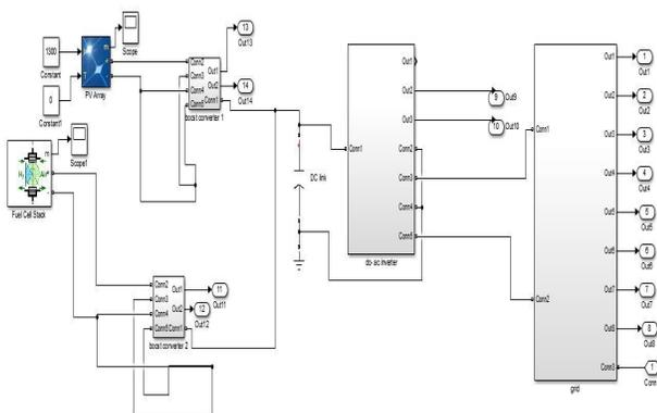
Fig. 4 Overall SIMULINK model of the proposed system
