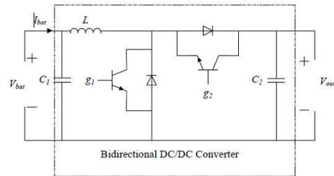
Fig 2 Bidirectional DC to DC Converter
