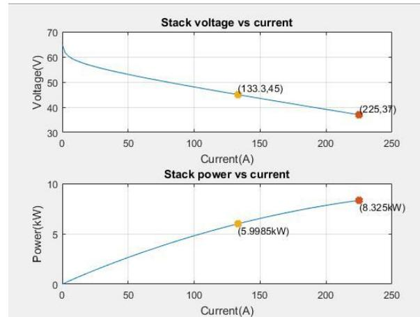
Fig 7 Voltage and Power Characteristics of Fuel Cell stack
