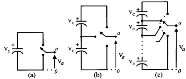
Fig.1.1 Single Phase Leg of an Inverter with (a) Two levels (b) Three levels (c) n-levels with different numbers of levels,
