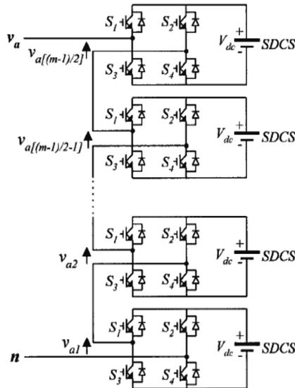
Fig 3.1 Single Phase Structure of a Multilevel Cascaded Inverter
