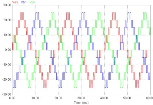
Fig 5.4 Three Phase Output Voltage Waveform of Eleven Level Cascaded Multilevel Inverter using additional switching
