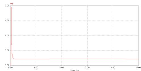
Fig 5.6 THD of Eleven Level Cascaded Multilevel Inverter using Additional Switching
