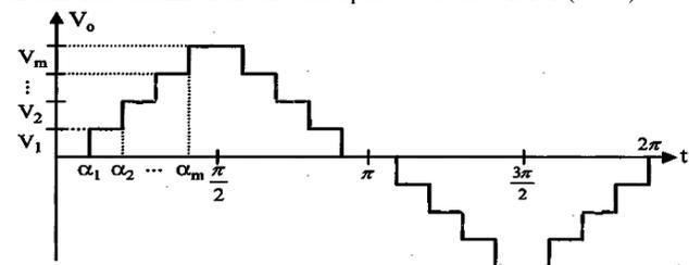
Fig 2.1 A generalized quarter-wave symmetric stepped voltage waveform synthesized by a  $(2m+1)$  – level inverter
