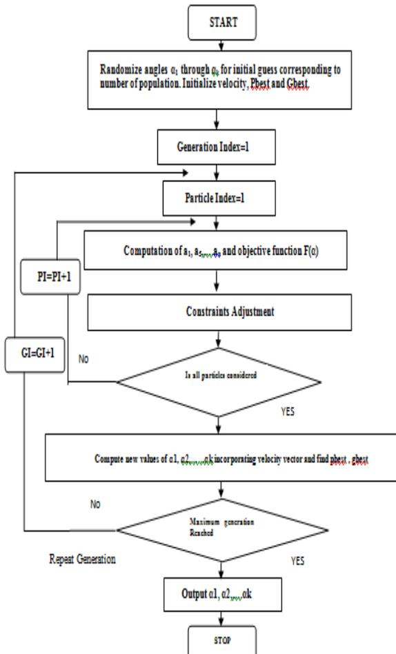
Fig 4.1 Flow Chart for PSO Algorithm
