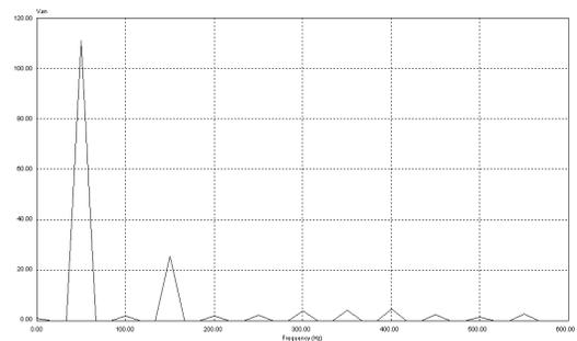
Fig 5.2 FFT Analysis of Seven Level Cascaded Multilevel Inverter using Additional Switching
