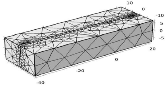
Fig. 2. Meshing results of the condenser T1
