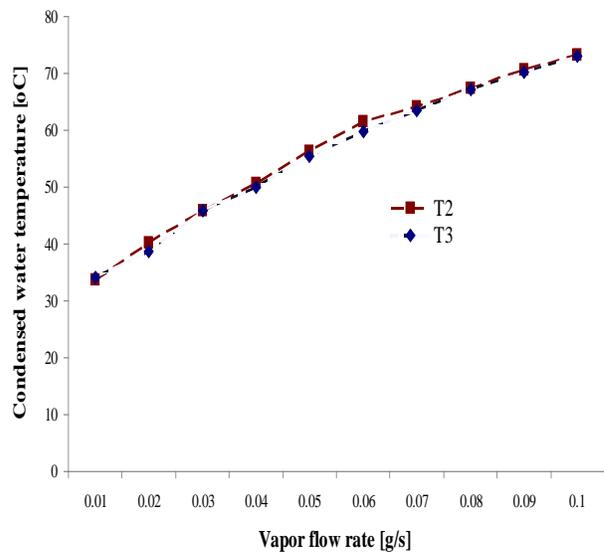
Fig. 7. Comparison between the condenser T2 and the condenser T3
