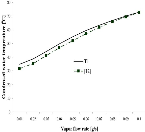
Fig. 4. Comparison between the condenser T1 and the condenser in [12]
