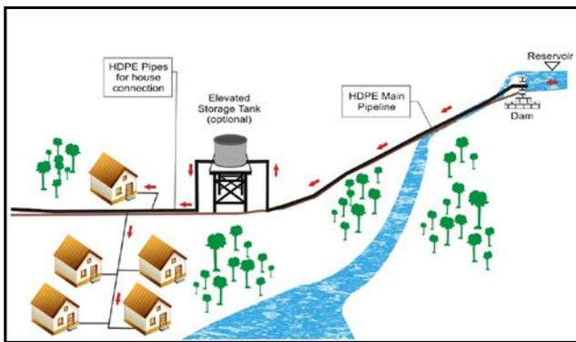
Figure 1.1 Schematic Diagram of Gravity Feed System (GFS) for Rural Water Supply
