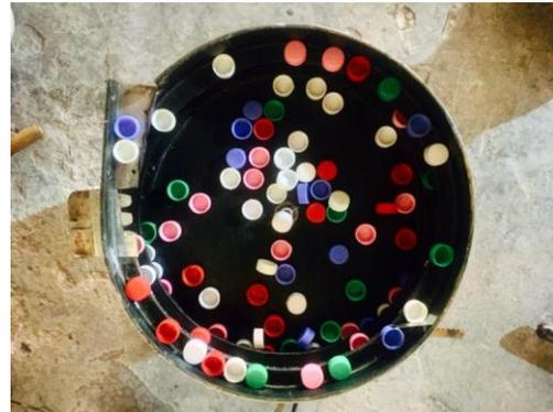
Figure 2: Bottle caps fed into the vibratory bowl feeder
