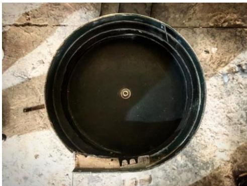
Figure 1: Vibratory bowl feeder (top view)
