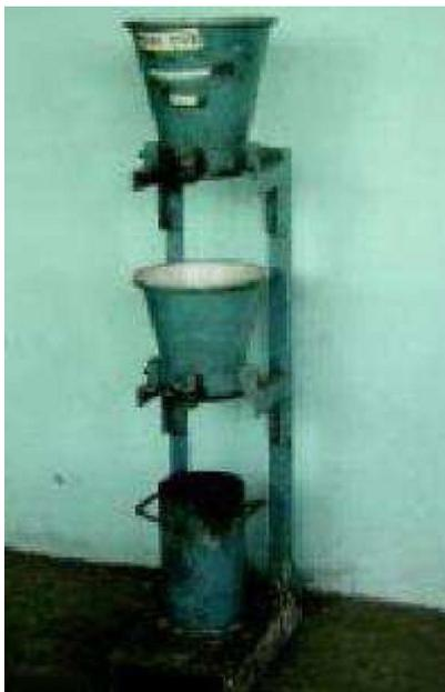
Fig2 Compaction factor test
