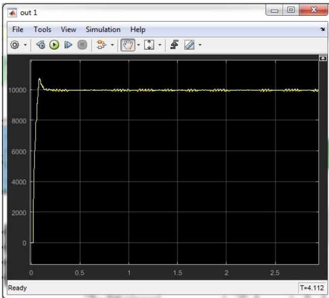
power output from hybrid model(solar wind MPPT)
