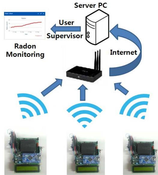
Fig. 1 Concept of Wi-Fi based radon monitoring
