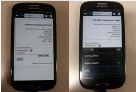
Fig. 5. Assigning of new SSID and password to a Wi-Fi router
