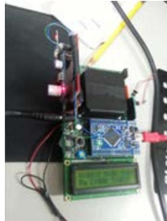
Fig. 4 ESP8266 Wi-Fi module connected to the implemented radon counter
