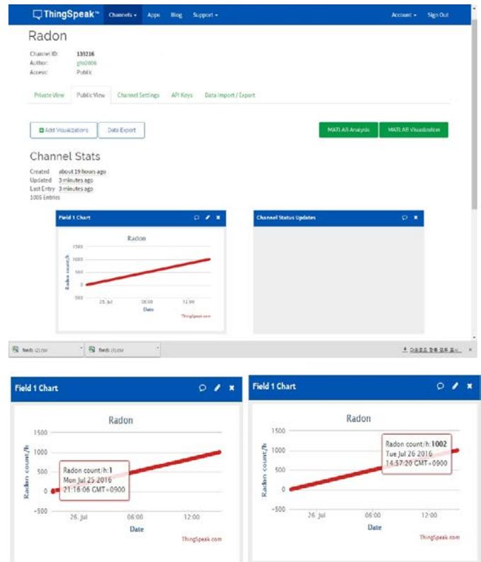
Fig. 9 Transmission test of a Wi-Fi system with an interval of 1 min, for 1000 times
