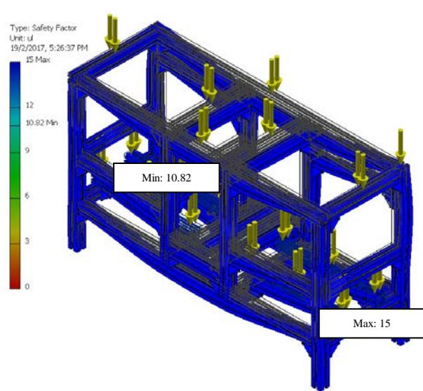
Fig. 10 Safety factor consideration based on bun machine subjected loading
