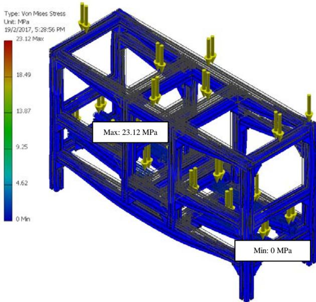
Fig. 8 Von Mises Stress of bun machine frame
