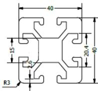
Fig. 3 Cross section of aluminum profile in mm
