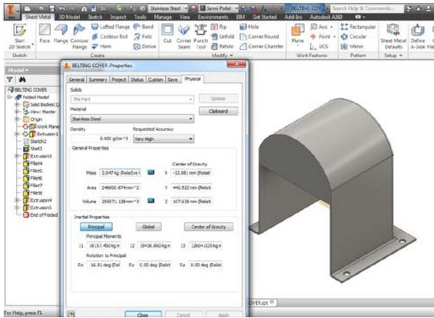
Fig. 6 Estimation load is base on prediction given by Autodesk Inventor software.
