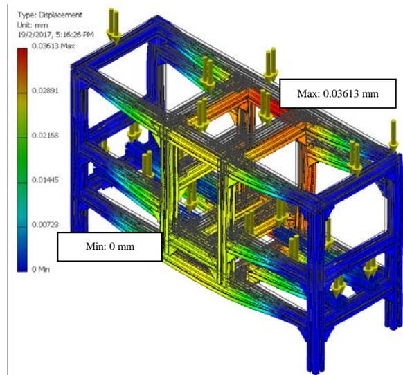
Fig. 9 Displacement on vertical axis of bun machine frame
