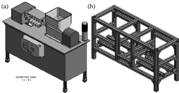
Fig. 2 Innovation of existing Bun Machine; (a) Complete assembly (b) Main Frame
