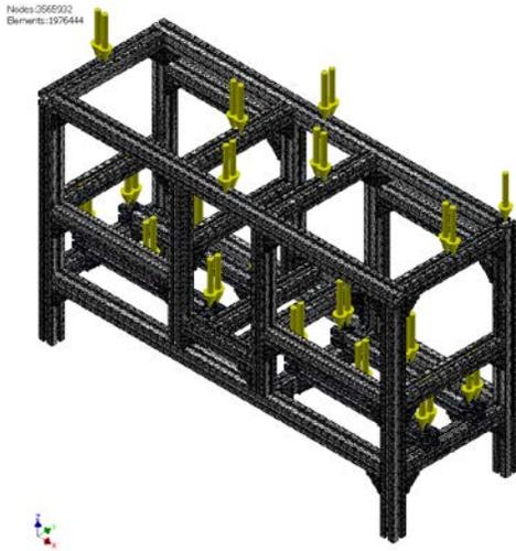
Fig. 7 Load that apply on frame
