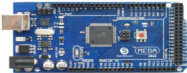
Fig.3 Arduino Mega2560
