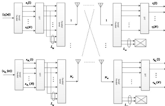
Figure1. MIMO-OFDM system model
