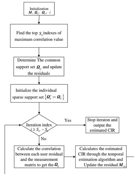
Figure4. JCE algorithm flow
