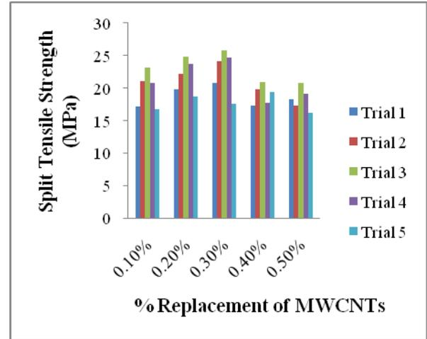
Fig.2 Comparison of split tensile strength of foam concrete specimens
