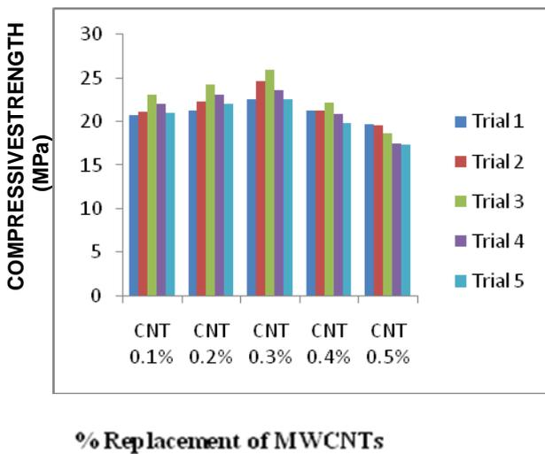
Fig.1 Comparison of compressive strength of foam concrete specimens
