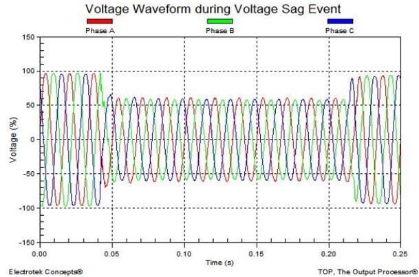
Figure 2.1 A Typical Voltage Sag Waveform
