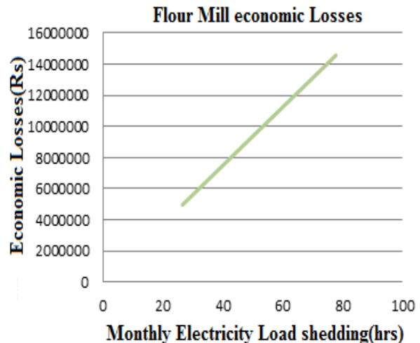
Fig. 4 Electricity load shedding Impacts on Economic Losses for Flour Mill
