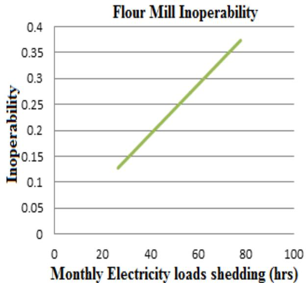
Fig. 3 Electricity load shedding effects on inoperability of Flour Mill.
