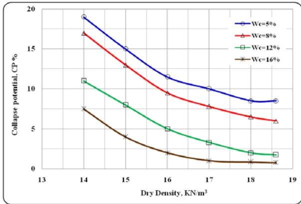
Fig. 6 Variation of collapse potential, with dry density
