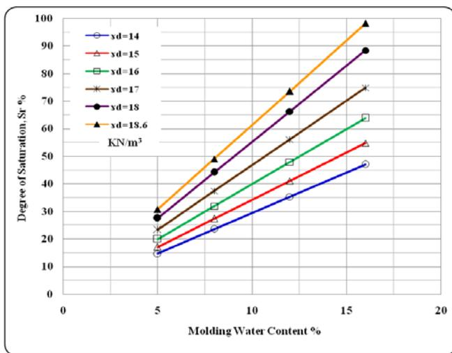
Fig. 10 Variation of degree of saturation, versus molding content.
