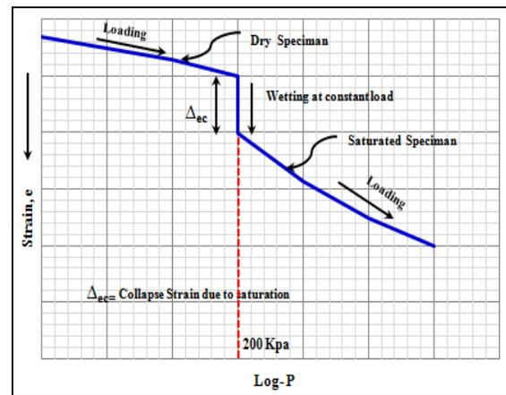
Fig. 2. Schematic diagram of single oedometer collapse test.
