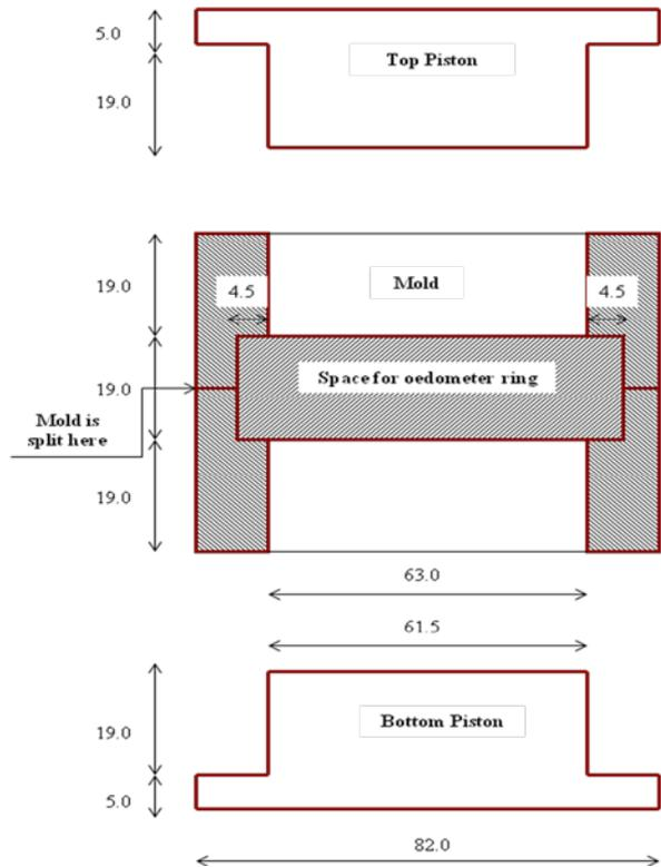
Fig. 4. Compaction mold. Dimensions in millimeters.
