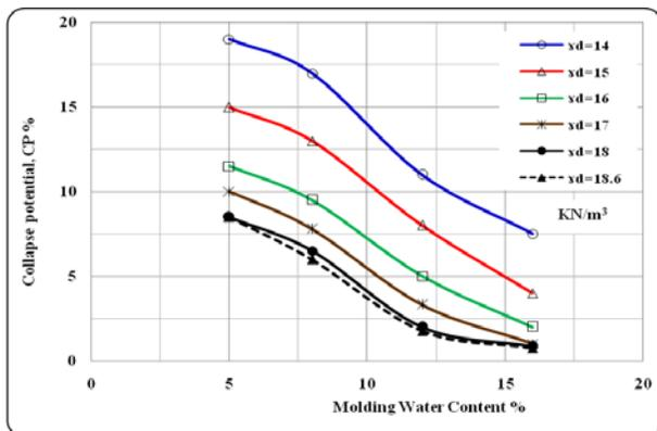
Fig. 7 Variation of collapse potential, with molding water content.
