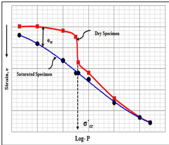
Fig. 3. Schematic diagram of double oedometer test.
