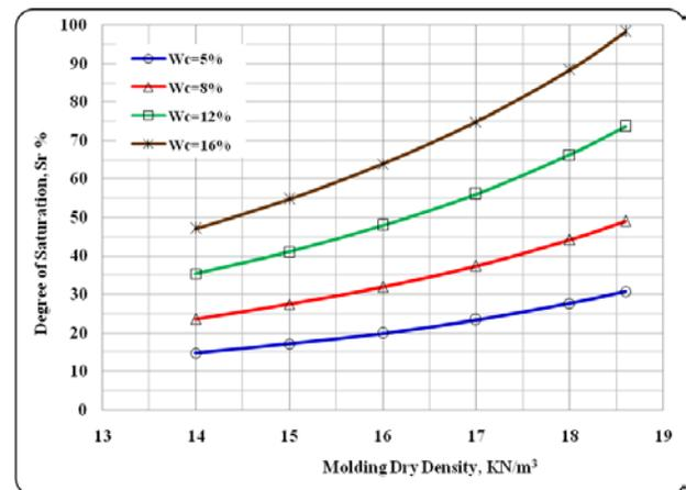
Fig. 9 Variation of degree of saturation, versus dry density.
