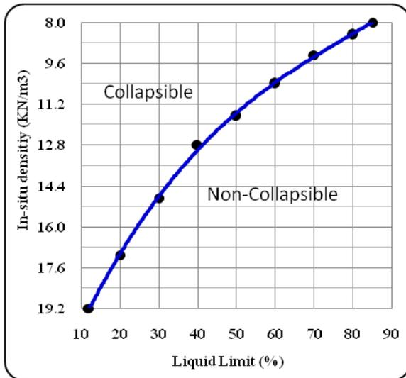
Fig. 1. Identification of collapsible plastic soils (After Gibbs and Bara, 1962 [19]).
