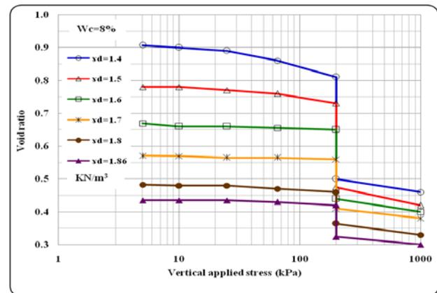
Fig. 5 Results of collapse tests for various compacted density at Wc=8%
