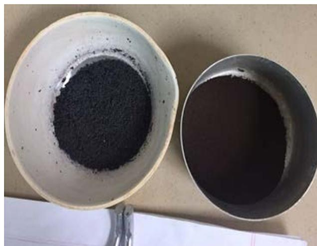
Fig 1: Sewage sludge ash out from the furnace (Left), pulverized sewage sludge ash (Right)
