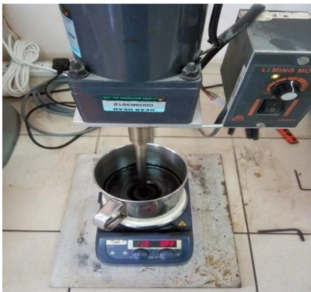
Fig 2: Mechanical mixer used to blend SSA with bitumen
