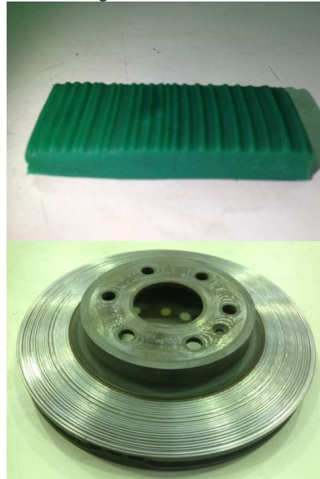
Figure 9: Grooved modified disc brake
