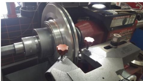
Figure 6: Brake lathe machine to reface the rotor
