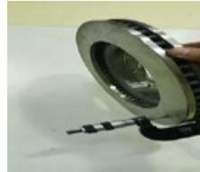
Figure 7: Micrometer to check the rotor thicknesses
