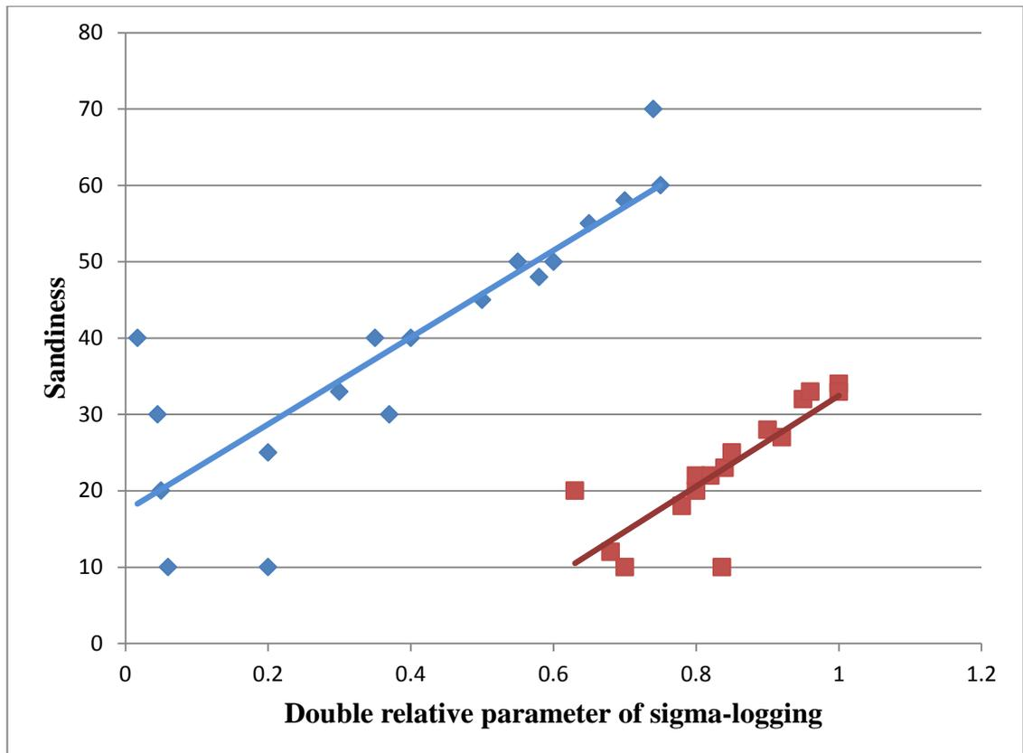
**Figure 2. The relation of the sandiness of rocks on the double relative parameter of sigma-logging:**
