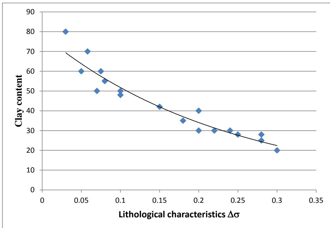
**Figure 1. The dependence of the clay content on the lithological characteristic  $\Delta\sigma$  of the complex of parameters of rock properties in the classification of the drill cuttings.**
