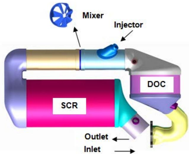
Fig. 7. SCR Inlet Cone Design Proposal 1.
