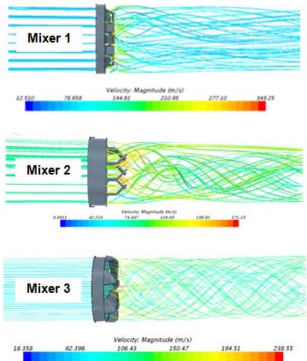
Fig. 5. Streamlines visualizing the effect on the flow field of three different mixers.
