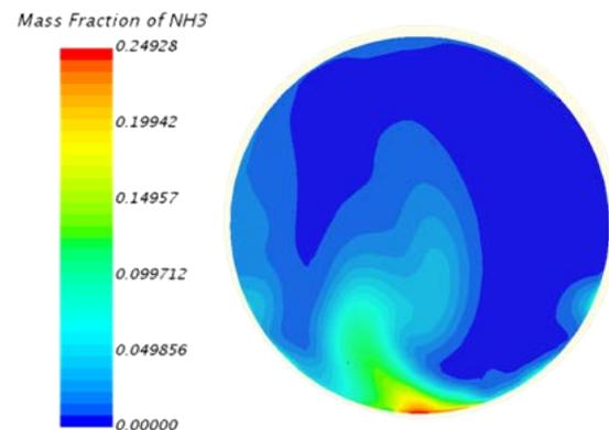
Fig. 8. CFD plot of NH<sub>3</sub> distribution for SCR Inlet Cone Proposal 1.
