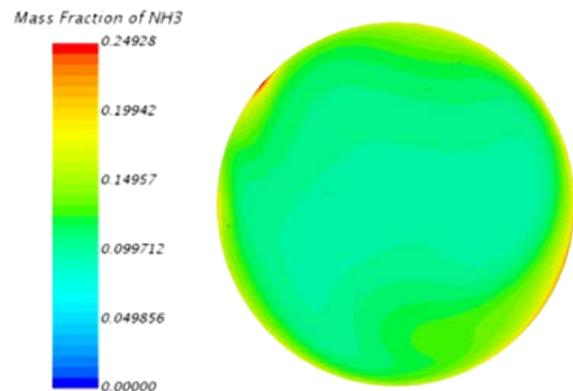
Fig. 11. CFD plot of NH<sub>3</sub> distribution for SCR Inlet Cone Proposal 2.
