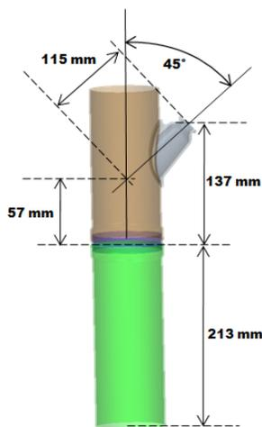
Fig 4. Intermediate mixing pipe for SCR.
