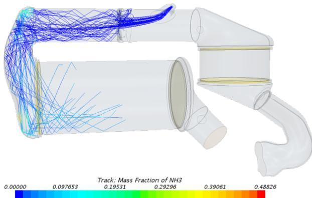
Fig.12. NH<sub>3</sub> particle distribution inside SCR Inlet Cone Proposal 2.
