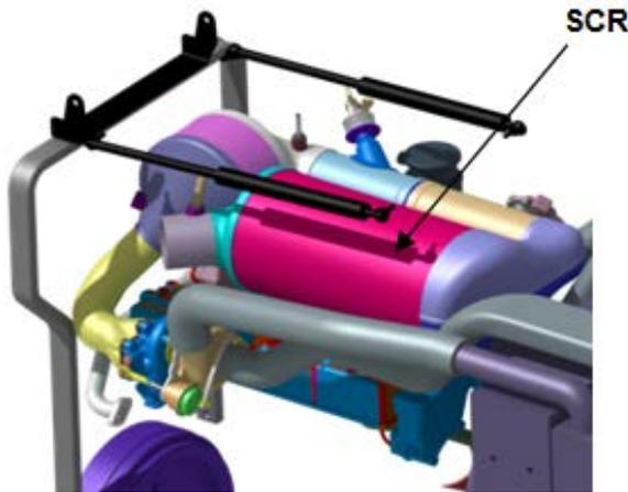
Fig. 2. SCR exhaust aftertreatment package.
