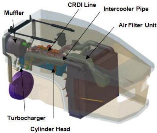
Fig. 1. Vehicle underhood parts in close proximity with SCR exhaust aftertreatment system.
