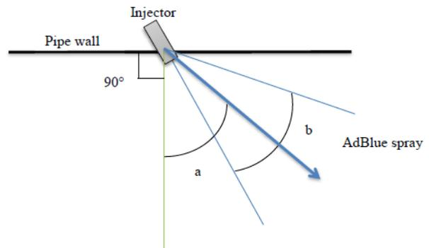
Fig. 3. A schematic figure of injector for the UWS sprays injection.
