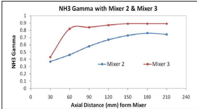
Fig. 6. Comparison of NH<sub>3</sub> gamma value for mixer 2 & 3.
