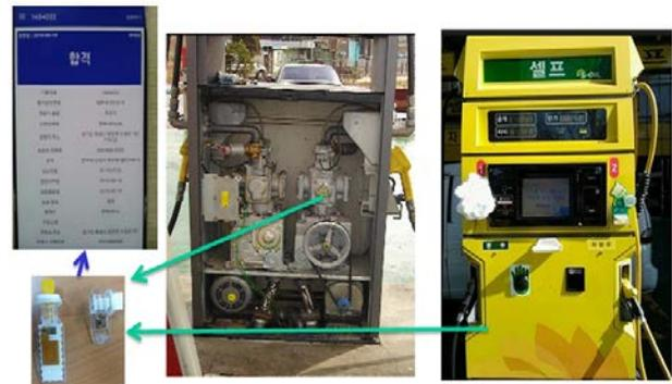
Fig. 6 NFC experimental system applied to oil lubricator seal device
