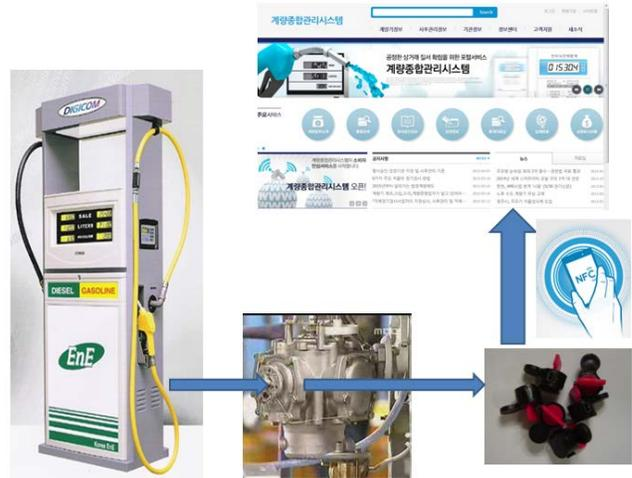
Fig. 1 Schematic diagram of NFC application to metrology seal device
