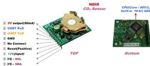
Fig. 3 Pin assignment of the NDIR CO<sub>2</sub> sensor H-550 (ELT, Korea).
