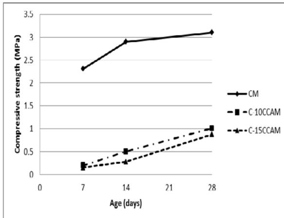
Figure 1: Effect of age on the compressive strength of PC/CCA mortar
