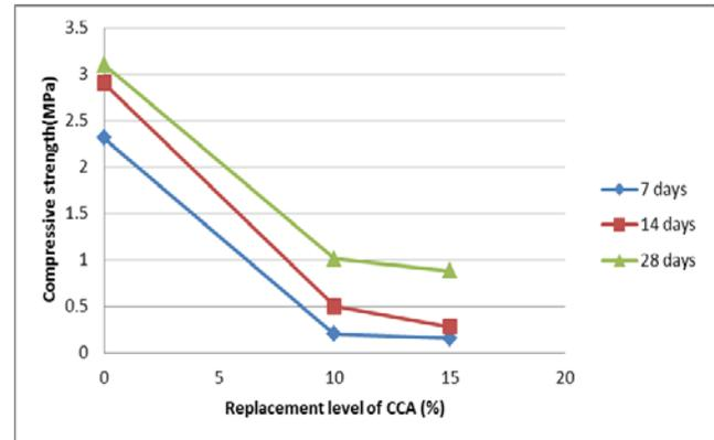
Figure 2: Effect of replacement level on the compressive strength of PC/CCA mortar
