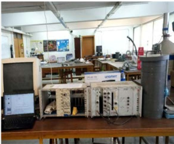
**Fig. 3:** Experimental set up for FJ374 NaI(Tl) scintillation detector
