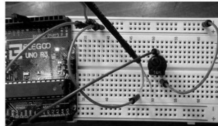
Fig. 2: Voltage Divider Circuit
