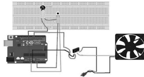
Fig. 1: Control System Schematic
