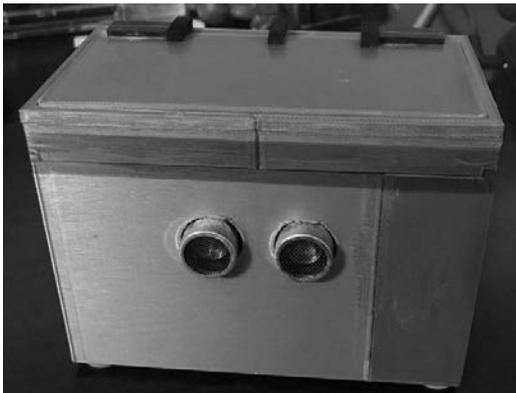
Fig.5: The Completed Assembly of the Tool Dispenser
