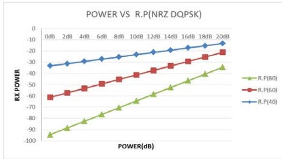
**Figure 7:** Powers vs. Received power
