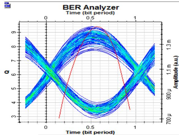
**Figure8(b):**Eye diagram analysis for 60Gbps DPSK-NRZ at user-1
