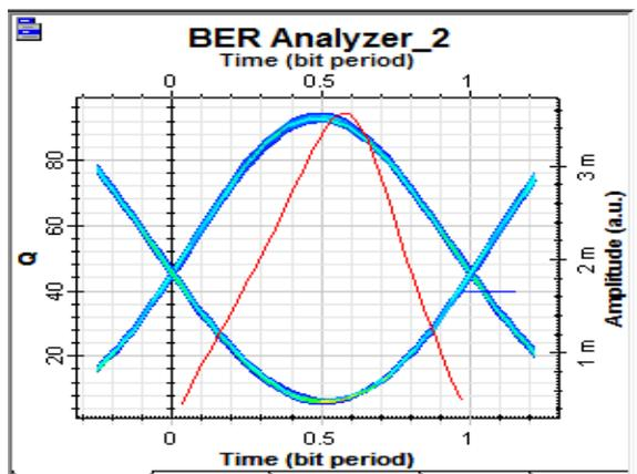
**Figure 8(a):**Eye diagram analysis for 40Gbps DPSK-NRZ at user-3. In this eye diagram it shows the quality factor of DPSK 40Gbps.
