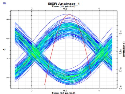
**Figure 8(c):** Eye diagram analysis for 80Gbps DPSK-NRZ at user-2
