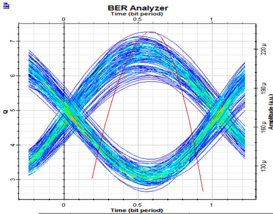
Figure9 (b): Eye diagram analysis for 60Gbps DPSK-NRZ at user-1
