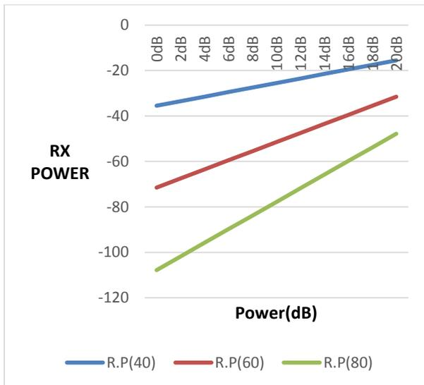
Figure 5: Power vs. Received Power
