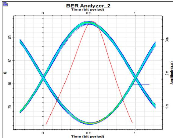
Figure9 (a): Eye diagram analysis for 40Gbps DPSK-NRZ at user-3
