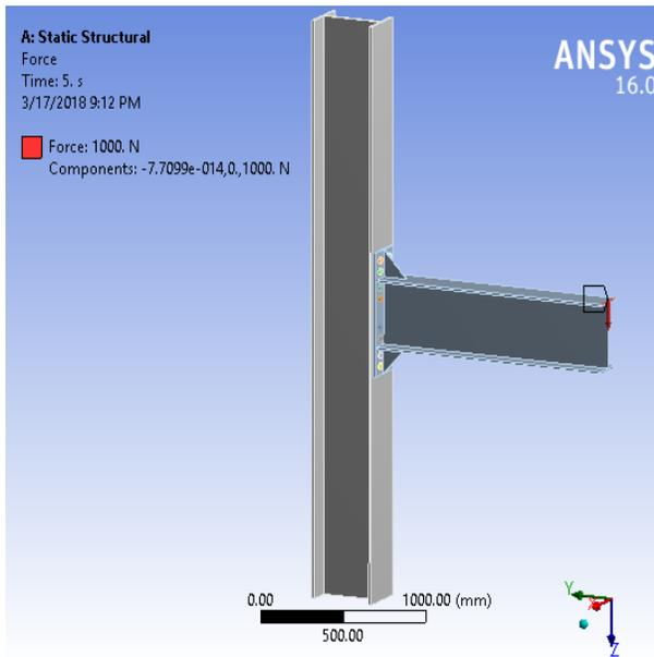
Fig 3 Loading at the tip of the beam and without pretensioning of bolts
