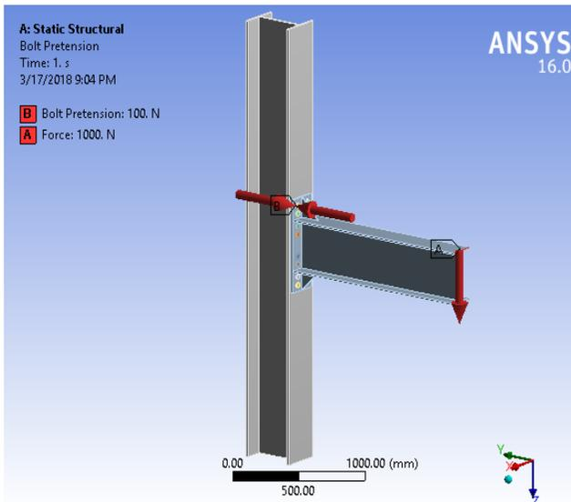
Fig 4 Loading at the tip of the beam and with pretensioning of bolts
