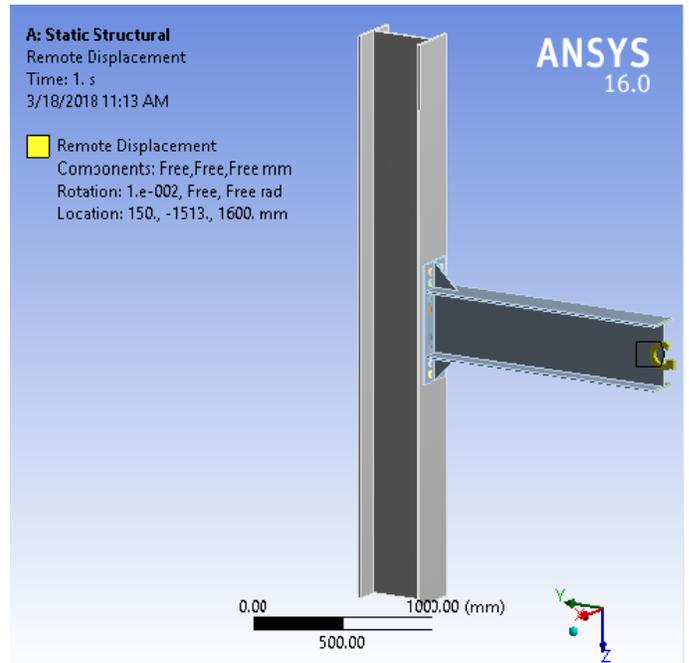
Fig 5 Cyclic rotations are applied at the end of the beam and without pretensioning of bolts
