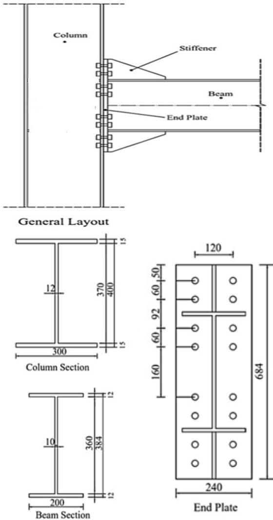
Fig 1 The details and geometrical dimensions of beam column joint
