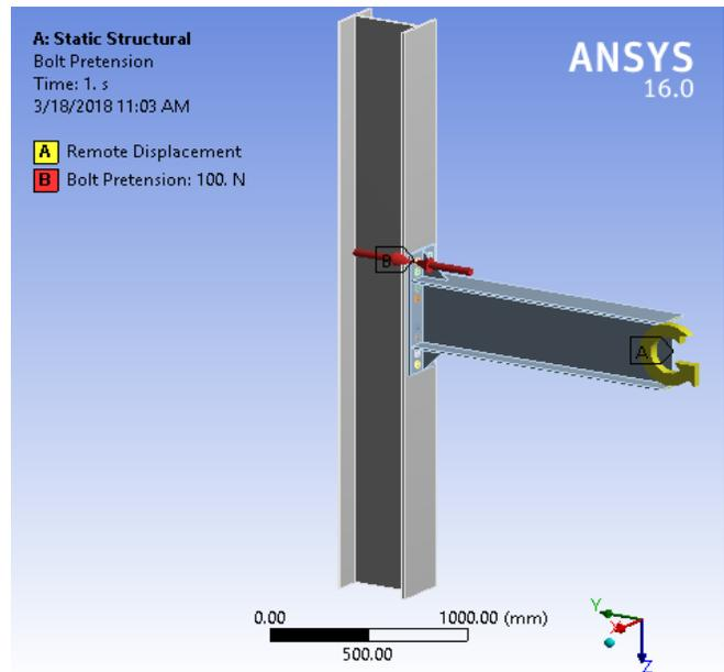
Fig 6 Cyclic rotations are applied at the end of the beam and pretensioning
