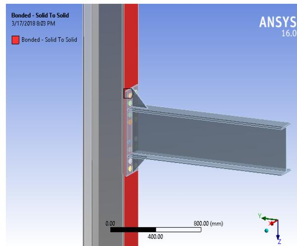
Fig 2 The model of beam column joint with filled rib
