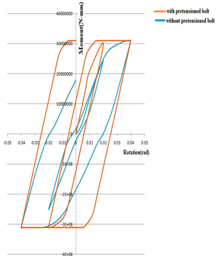
Fig 7 Moment –rotation graph for steel beam-column joint
