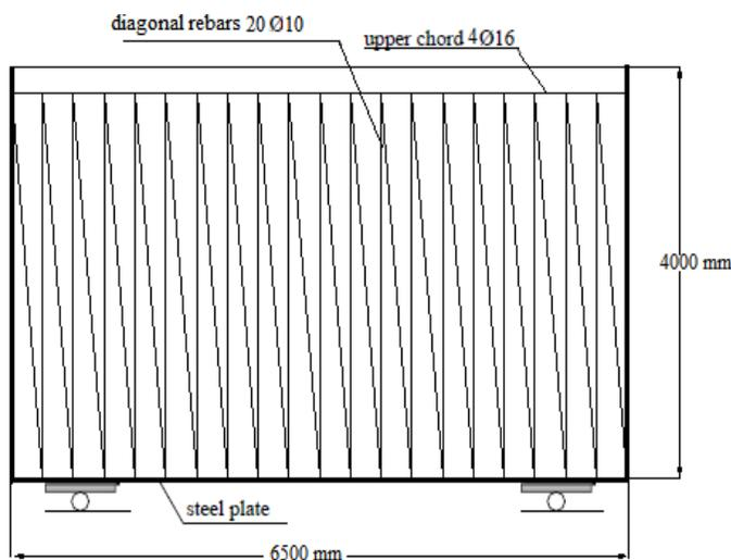
Fig. 2 Sectional drawing of steel trussed deep beam
