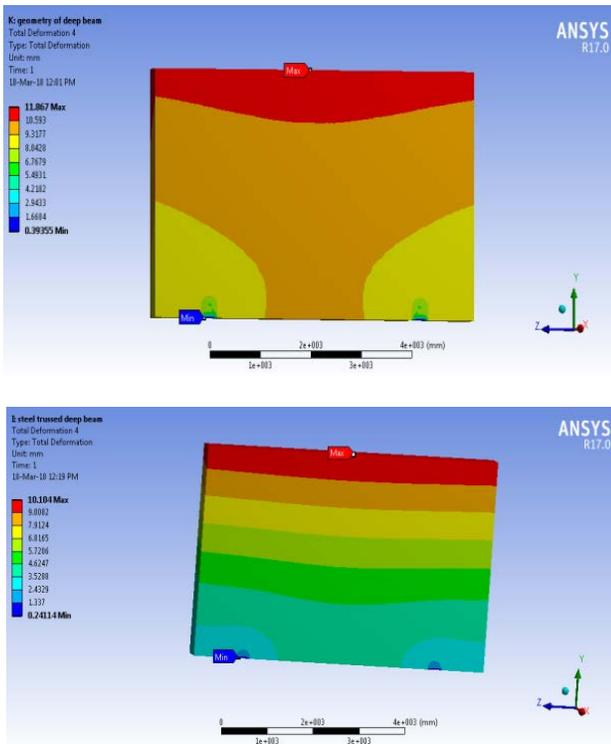
Fig. 4 Total deformation of conventional deep beam and hybrid steel trussed concrete deep beam
