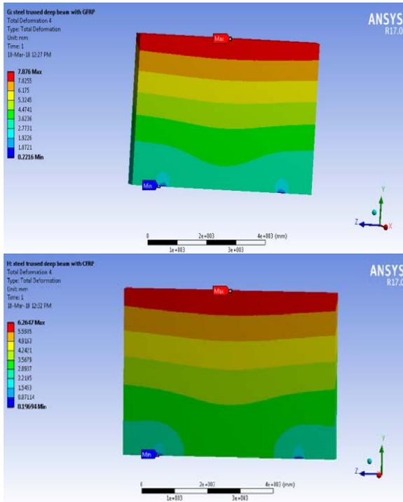
Fig. 7 Total deformation of hybrid steel trussed concrete deep beam with GFRP and CFRP
