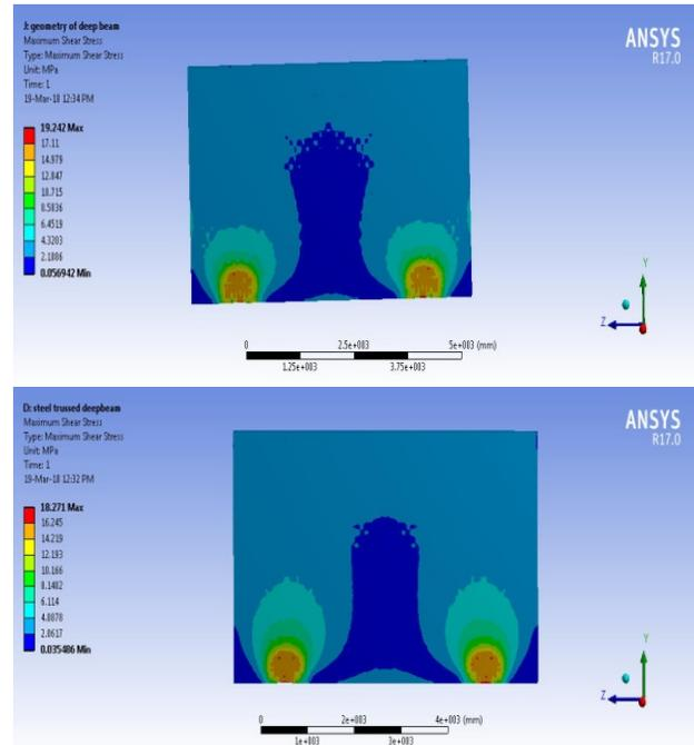
Fig. 5 Shear stress of conventional deep beam and hybrid steel trussed concrete deep beam
