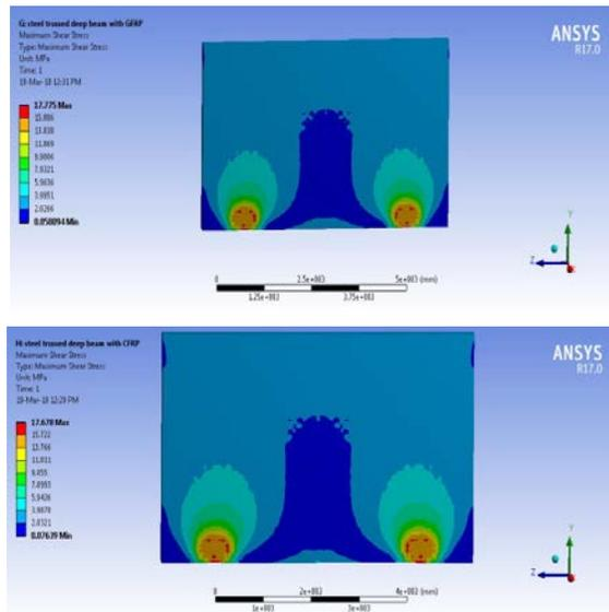
Fig 8 shear stress of hybrid steel trussed concrete deep beam with GFRP and CFRP
