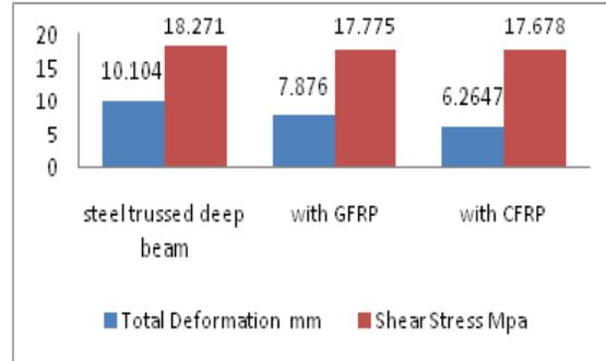
Fig.9. comparison of results of total deformation and shear
