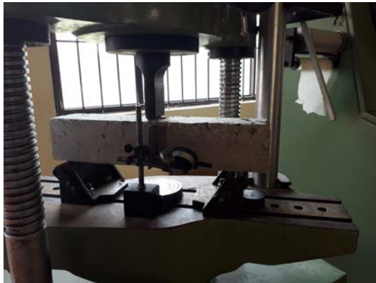
Fig. 6. Test setup for three point bending
