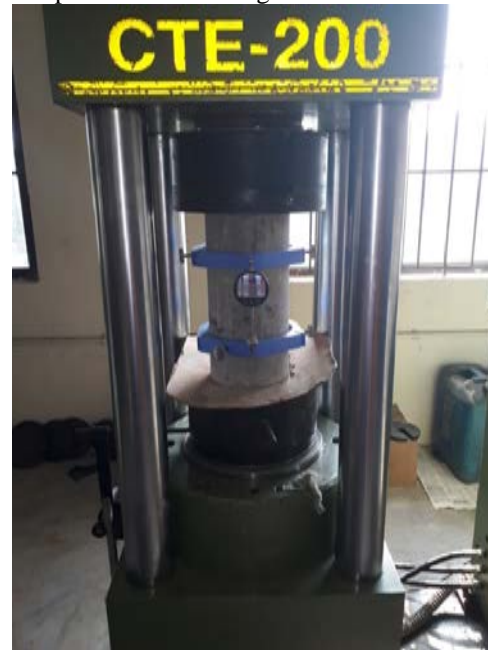
Fig. 5 Test setup for finding modulus of elasticity
