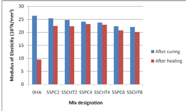
Fig. 5. Variation of modulus of elasticity at 28 days of curing and after healing of specimen having sodium silicate as healing agent
