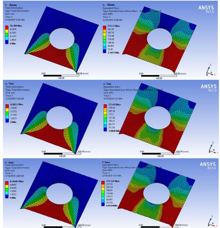
Fig.9 .Deformation and stress diagram of SPS with 6, 7mm and 8mm thick inner core
