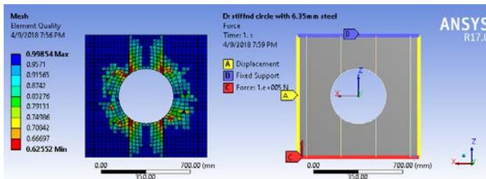
Fig.3 Meshing and loading diagram in ANSYS
