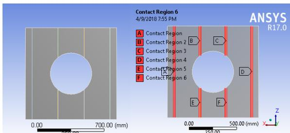
Fig.2 Geometrical modelling and contact between stiffeners and the surface body in ANSYS
