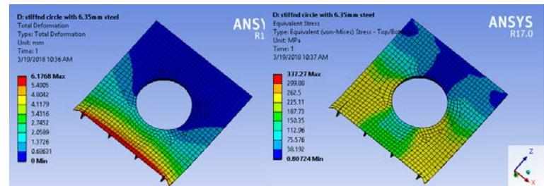
Fig.4 Deformation and stress diagram of steel plate with stiffeners
