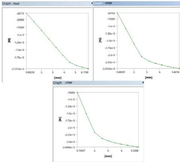
Fig.7 Load Deformation graph of steel, GFRP and CFRP sections
