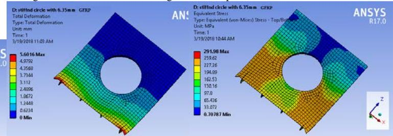
Fig.5 Deformation and stress diagram of GFRP plate with stiffeners
