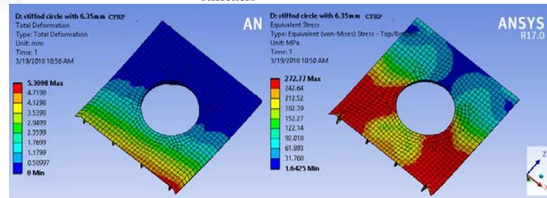
Fig.6 Deformation and stress diagram of CFRP plate with stiffeners
