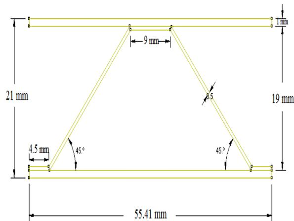
Fig. 1 Section details
