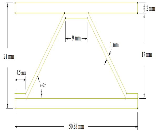
Fig. 2 Revised section details
