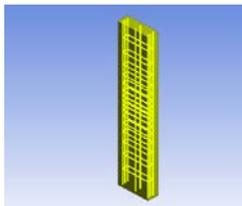
Fig.3 Reinforcement detailing of column model 2
