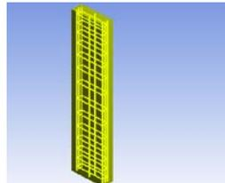
Fig.4 Reinforcement detailing of column model 3
