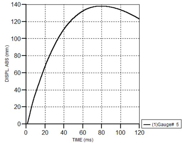
Fig. 11 Displacement Vs Time graph of column model 1
