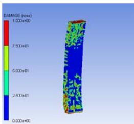
Fig. 14 Damage profile of column
