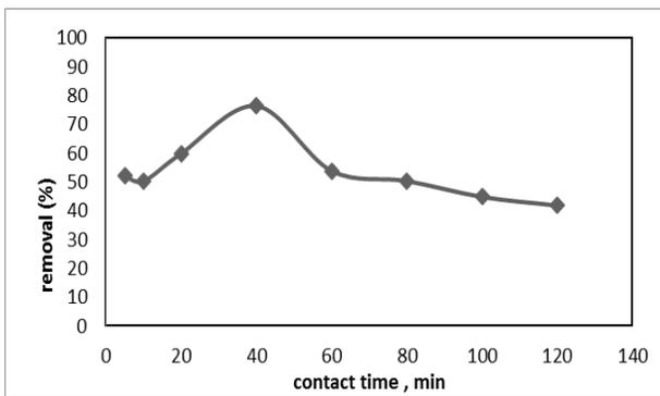
Fig3- The effect of contact time on chitosan absorption capacity in nitrate contaminant removal
