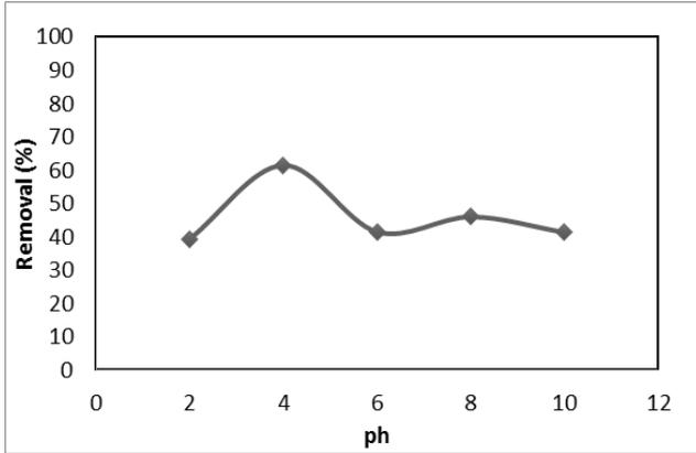
Fig1- Effect of pH on chitosan adsorption capacity in nitrate pollutant removal
