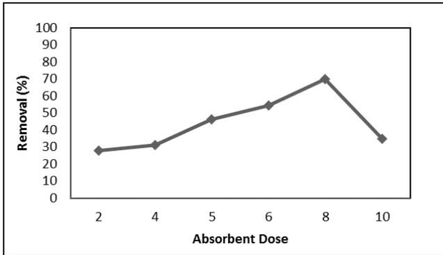
Fig 2- Effect of Adsorbent on Chitosan Adsorption Capacity in Removal of Nitrate
