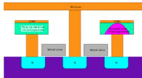
Figure 1: Fabrication structure of PRAM
