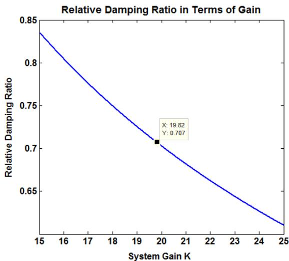
Figure 2. Gain value corresponding to relative damping ratio  $\zeta = 0.707$
