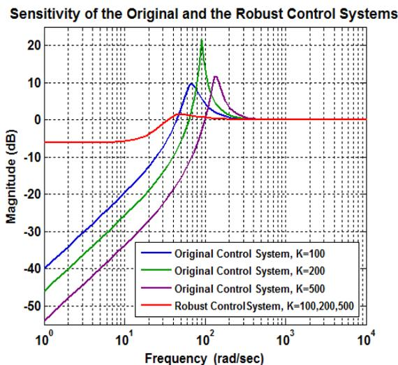
Fig.7. Sensitivity of original and robust control system (Variable gain  $K$ )
