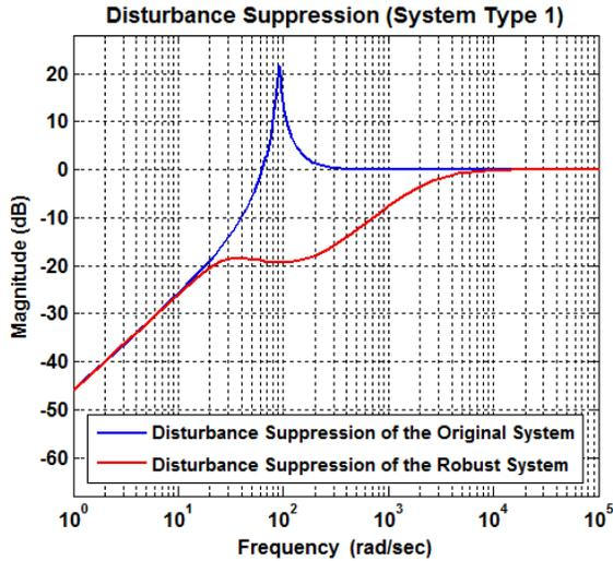
Fig. 8. Disturbance suppression of the original and robust control systems
