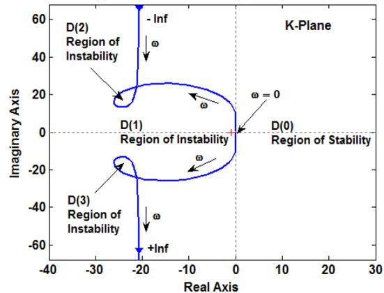
Fig. 4. D-Partitioning in Terms of  $K$  with the Robust Controller
