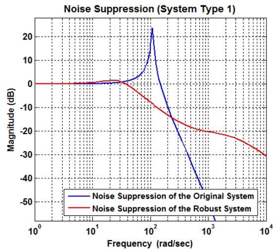
Fig. 9. Noise suppression of the original and robust control systems
