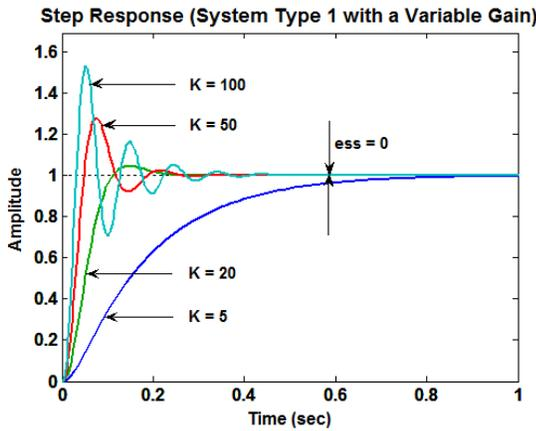
Fig. 5. Step responses of the original system with a Variable Gain
