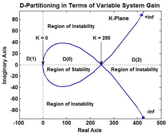
Fig. 3. D-Partitioning in terms of the variable system gain
