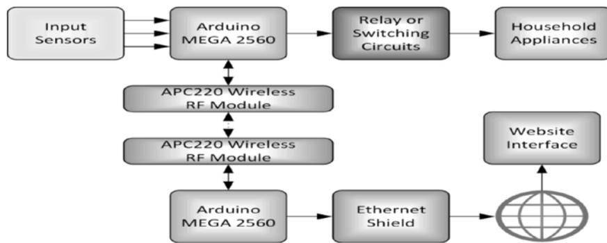
Fig.1 Block Diagram of Smart Home Control System(SHCS)
