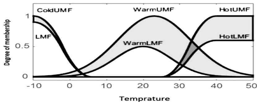
Fig.9 Temperature membership function
