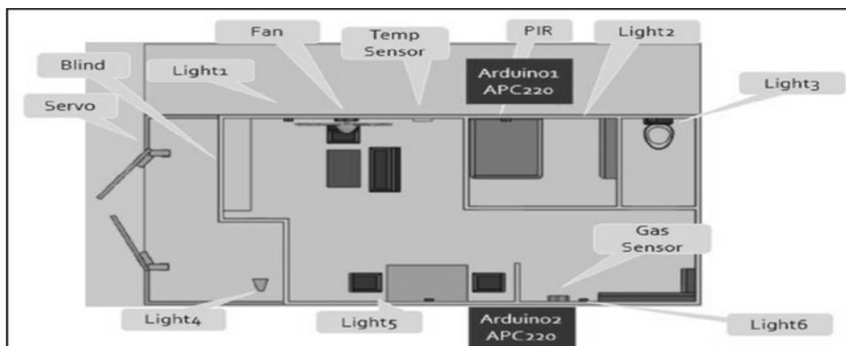
Fig.3 The top view of test field
