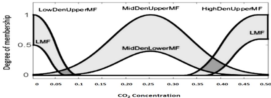
Fig.11 CO<sub>2</sub> concentration membership function
