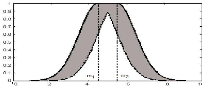
Fig.7 FOU for Gaussian (primary) MF with uncertain mean
