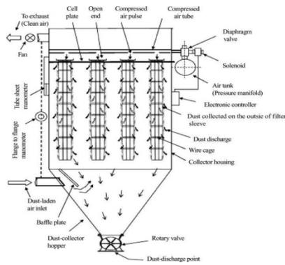
Residue loaded air-encouraging zone, Filter unit, Dust transfer framework, Fan (air mover) and release stack, Air store, Connecting funnels, Diaphragm valve, Blow pipe, Nozzles, Venturi-spout, Filter pack and enclosure get together, Bag channel lodging, Auxiliary connection, Safety highlights for touchy or inflammable residue.
