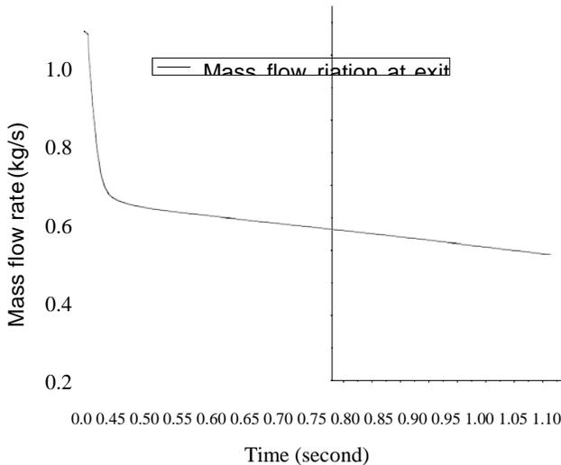
Figure 4.1 Mass flow variations in the reservoir 1 for blow tube with 12 nozzles.
