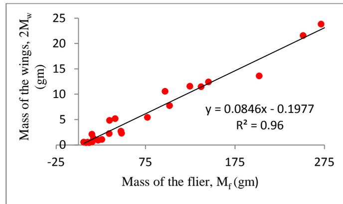
Fig.1. A plot between Mass of the wings and Mass of the flier
