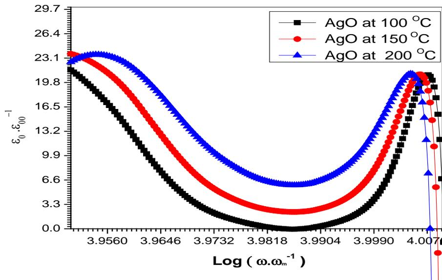
Fig.(3):Scaling behavior of ( $\epsilon_{00}$ )at various temperatures for Ag Oat 100, 150, 200 °C.
