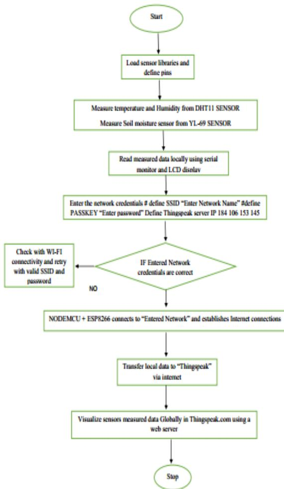
Fig. 4 Software implementation flowchart
