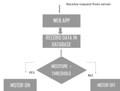
Fig. 3 Process flow for irrigation
