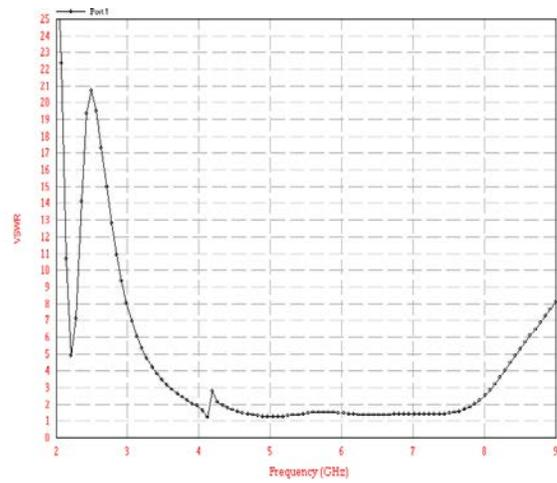
Fig. 4: Voltage standing wave ratio (vswr) Vs frequency
