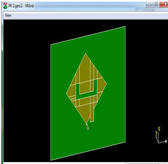
Fig. 2: 3D Geometry of irregular Diamond slotted antenna on IE3D
