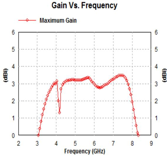
Fig. 9: Gain (dBi) Vs Frequency of microstrip patch radiator
