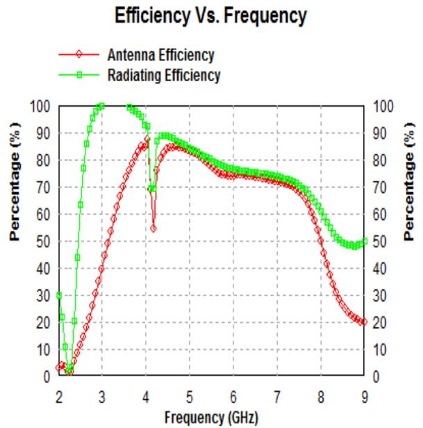
Fig. 11: Efficiency (Antenna and Radiating) Vs Frequency of microstrip patch radiator
