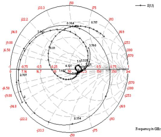
Fig. 5: Smith chart of proposed microstrip antenna
