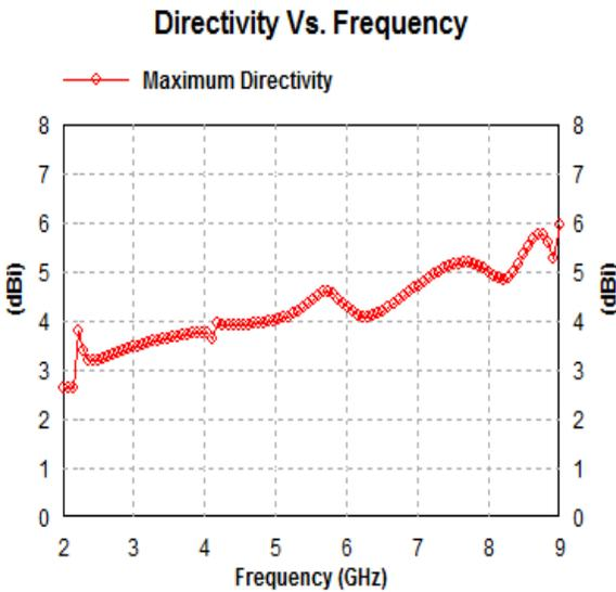
Fig. 10: Directivity Vs Frequency of microstrip antenna
